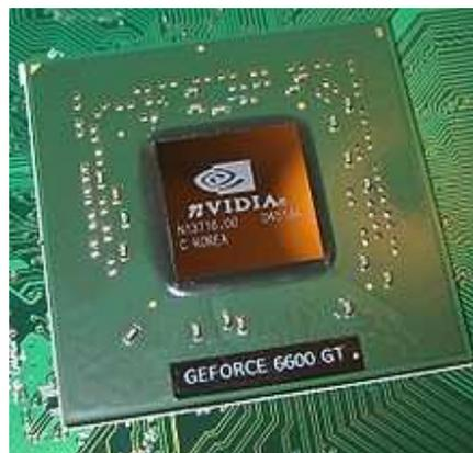
Fig 8 A GeForce 6600 GPU
